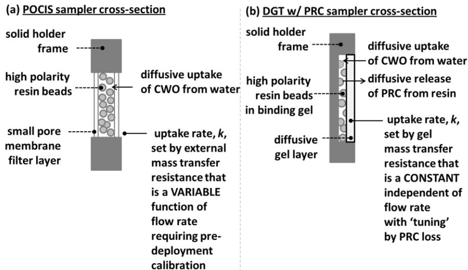
**Figure 1.** Schematic cross-section profiles of passive samplers noting the location of limiting mass transfer steps and the consequent influence on the sampler uptake rate,  $k$ , that is critical to calculating time-averaged aqueous concentrations (Eq. 1). Sampler length 5-8 cm.
