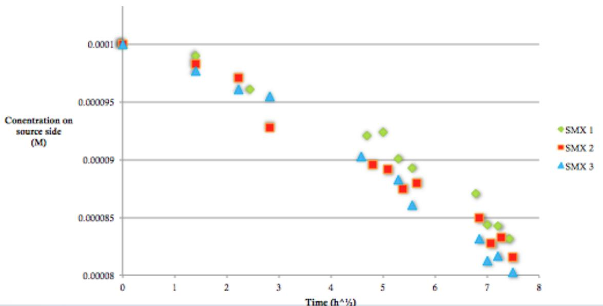
**Fig. 2.** Sulfamethoxazole transport from the ‘high concentration’ reservoir for duplicate subsamples of a single gel sheet (SMX-1 green diamonds, SMX-2 red squares) and from a duplicate gel sheet (SMX-3).
