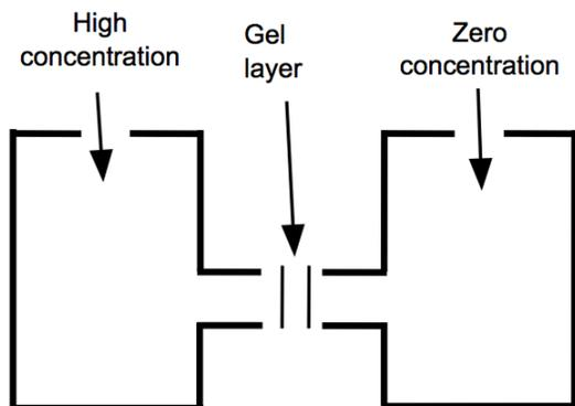
**Fig. 1** Diagram of diffusion cell used to obtain data for compound diffusion through the agarose gel material. Compounds moved from left to right in response to a diffusion gradient from high concentration ( $1 \times 10^{-4}$  M) to zero concentration (high purity water).
