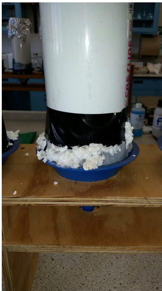
Figure 4. Crystals forming around base of columns with resin present, presumed to be NaOH.
